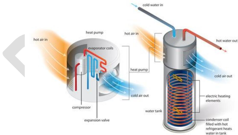
Figure 9: Schematic diagram of a Heat Pump Water Heater (Source: DOE ND)
