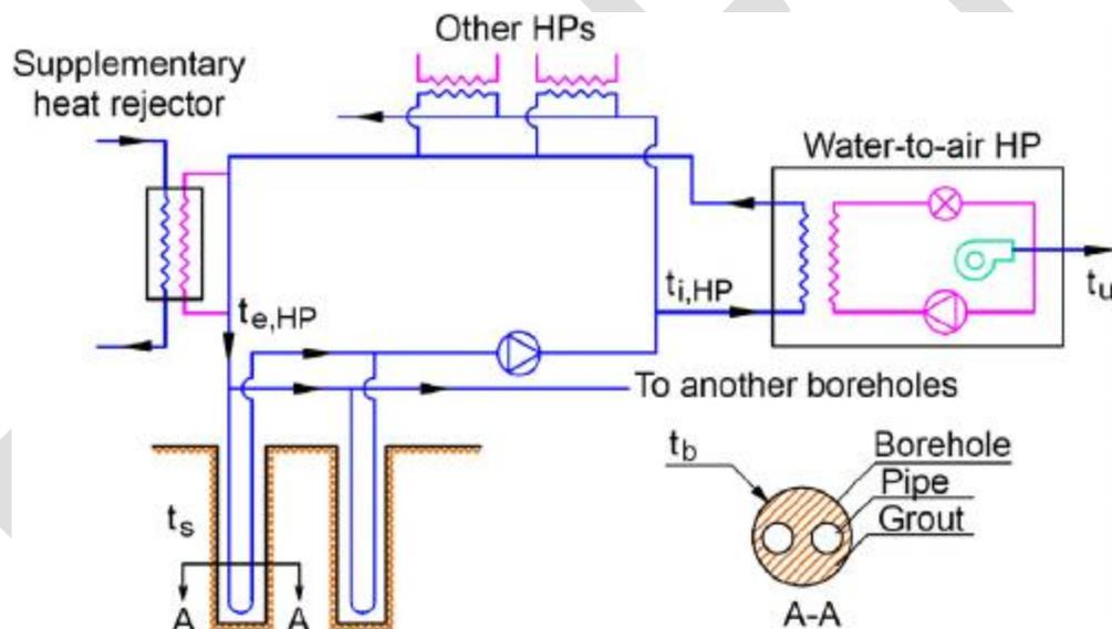
Figure 13: Schematic diagram of a closed-loop GSHP with vertical bore ground heat exchanger (Source: Sarbu and Sebarchievici 2013)
