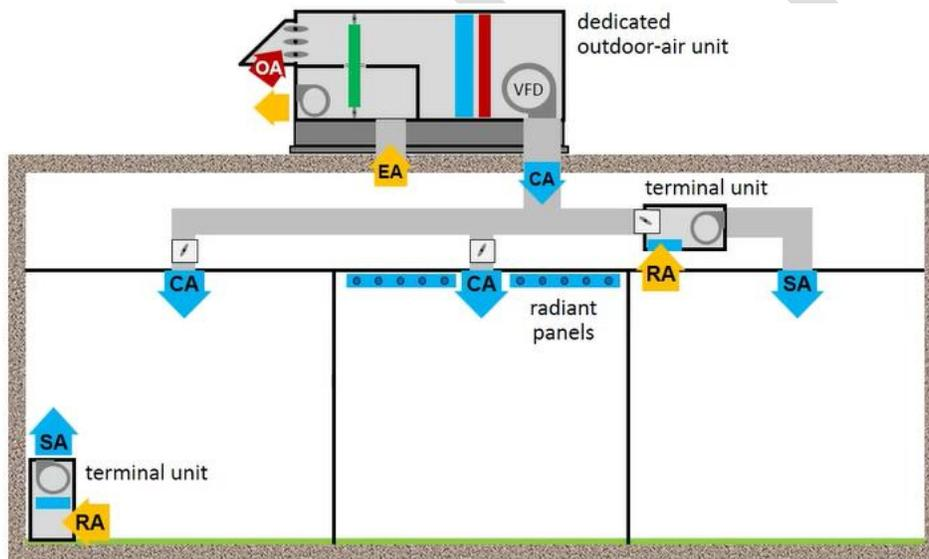
Figure 3: Diagram of a typical DOAS system
