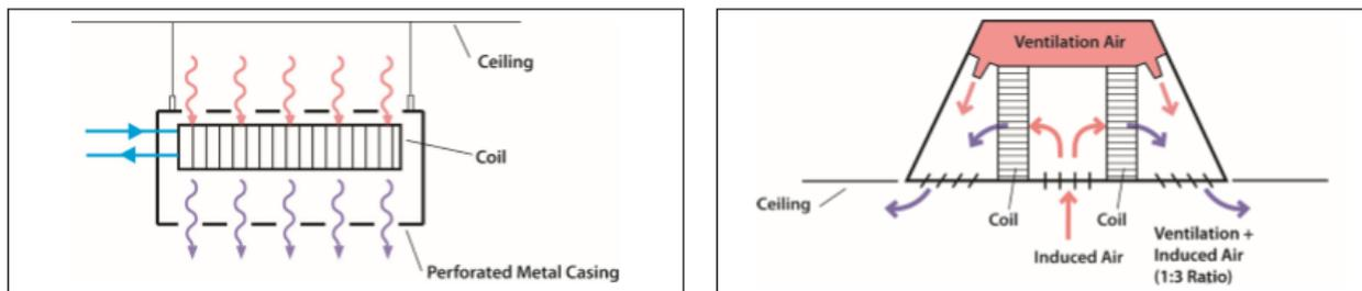
Figure 7: Schematic diagram of passive chilled beams (left) and active chilled beams (right)
