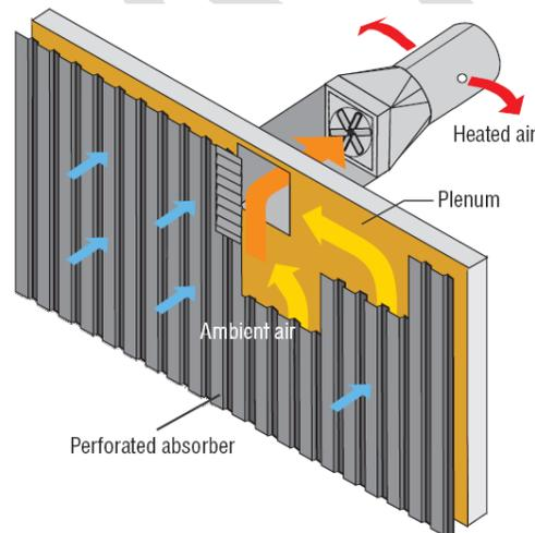
Figure 8: Schematic diagram of Transpired Solar Collector
