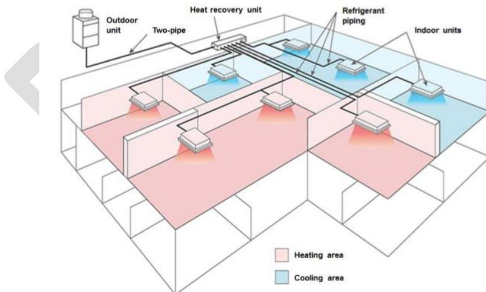
Figure 5: Schematic diagram of a VRF system
