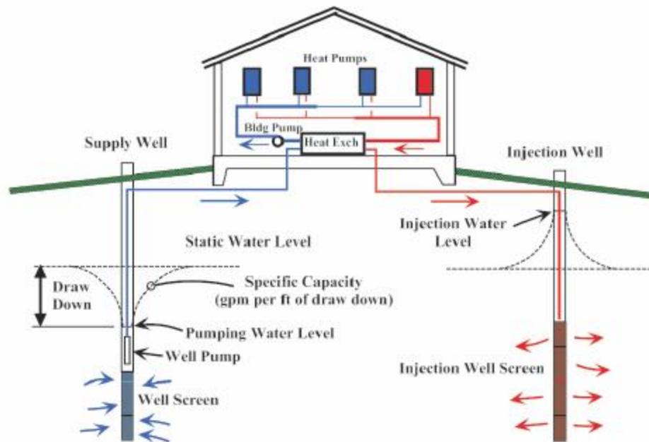
Figure 11: Schematic diagram of an open loop ground source heat pump with isolation heat exchanger (Source: Kavanaugh and Rafferty 2014)
