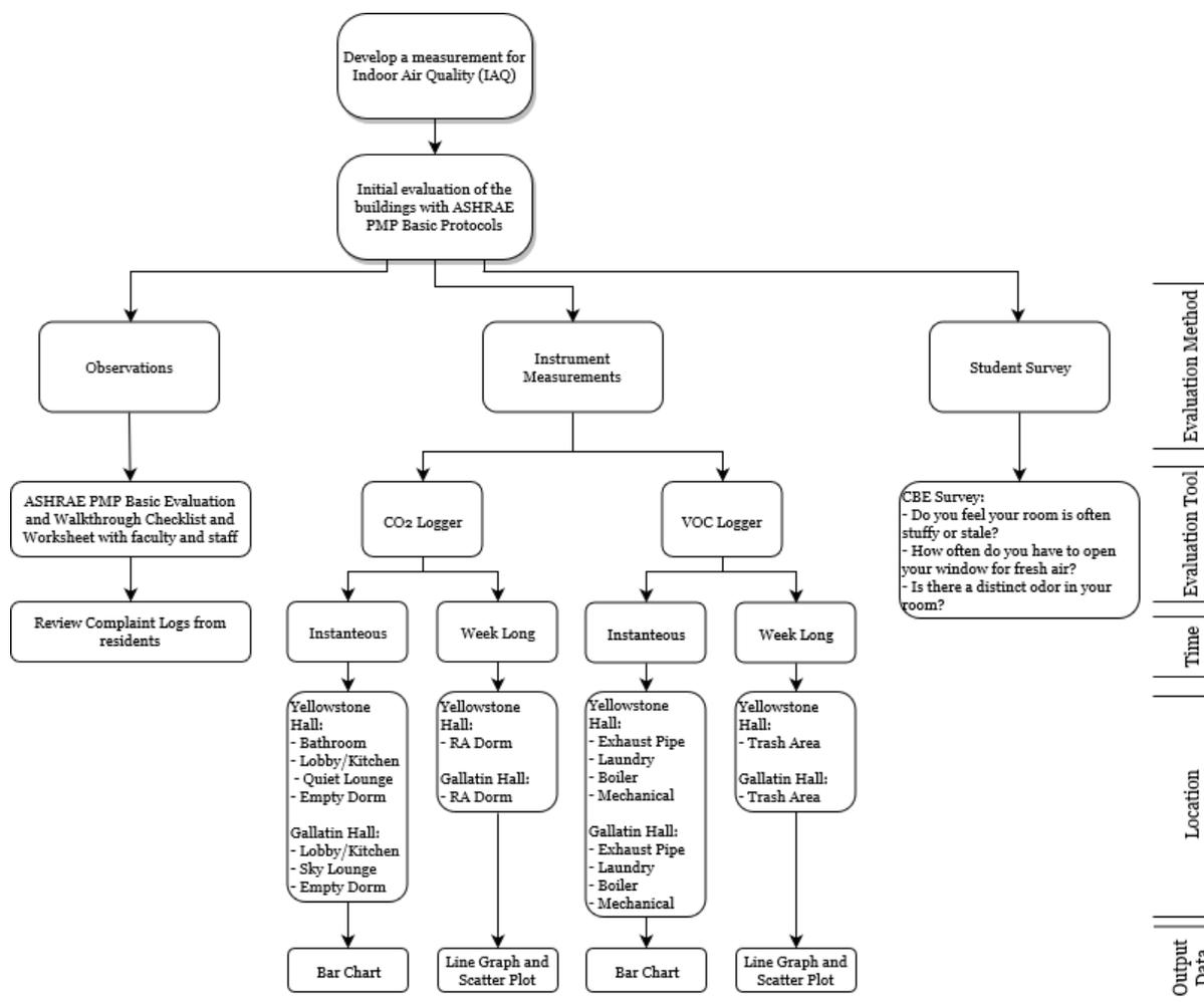
Figure 6: Flowchart indicating the use of ASHRAE PMP for evaluating IAQ conditions
