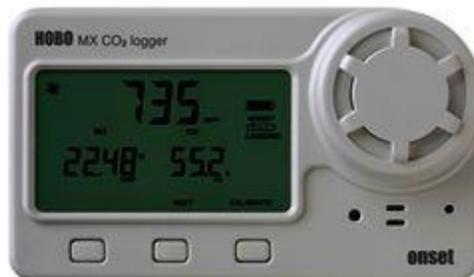
Figure 13: MX1102 HOBO Indoor Air Quality Logger
