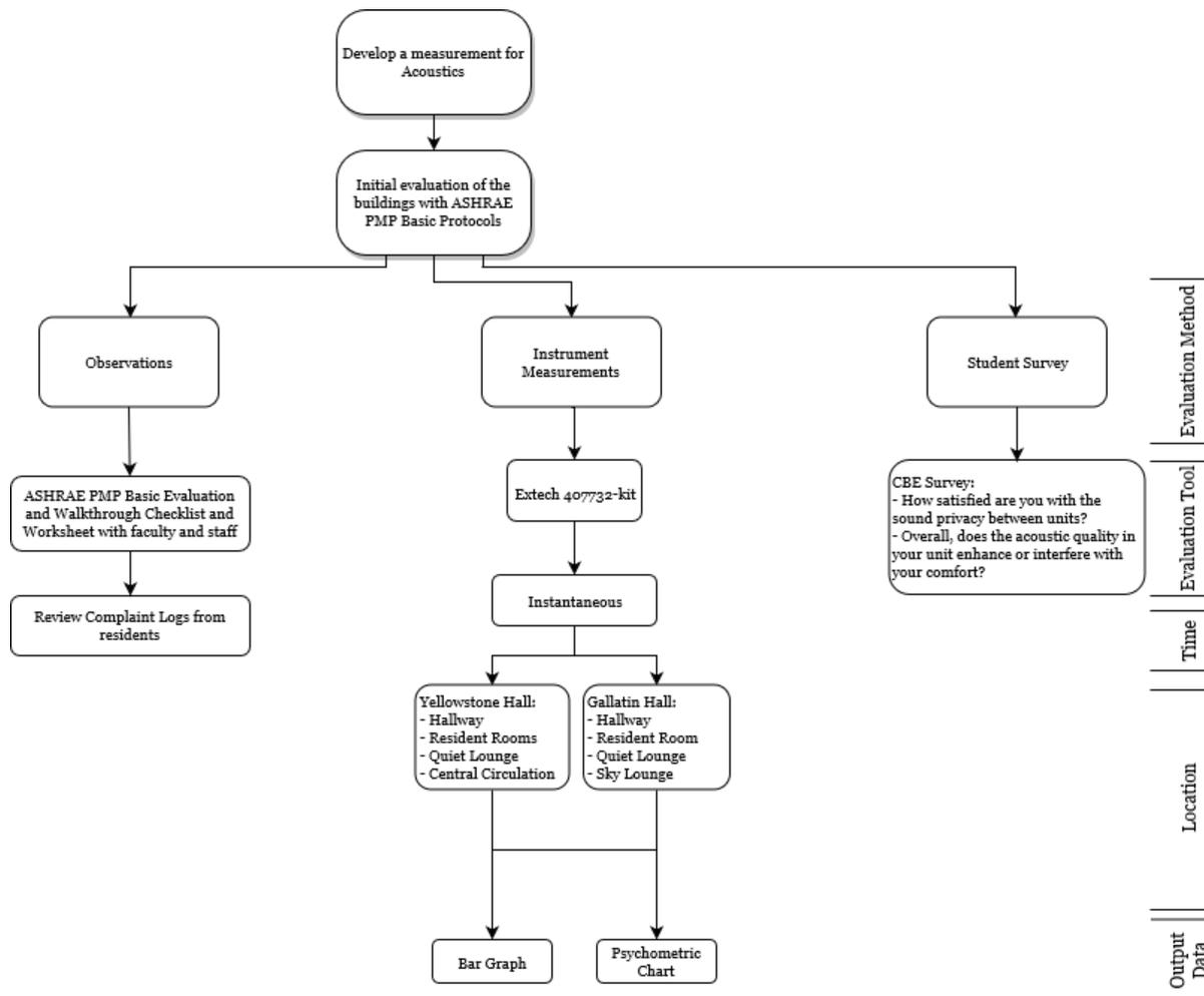
Figure 4: Flowchart indicating the use of ASHRAE PMP for evaluating acoustical conditions
