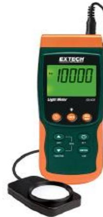
*Figure 12: Extech SDL400 Light meter device (right) used in the measurement of lighting levels*
