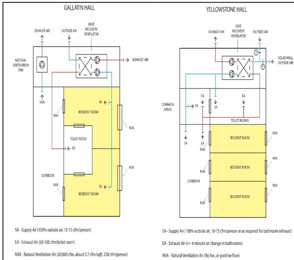
Figure 2: HVAC Diagrams for Gallatin and Yellowstone Halls
